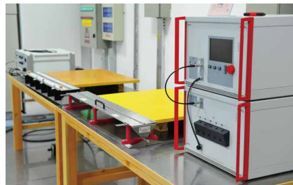
EMC surge testing
